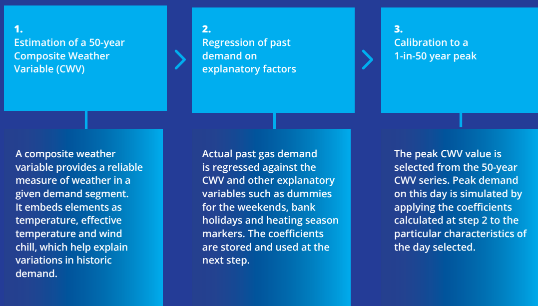
Figure 6: Procedure for estimating peak year gas demand
