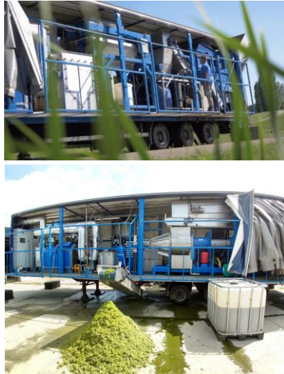
Figure 12: Mobile, containerised grass biorefinery plant. Source: biorefineryglas.eu
